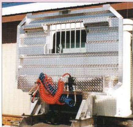
C. Standard upright cabguards available with optional window, chainhangers, and trays. 6" "I" - Beam mounting sills are the strongest in the industry.
