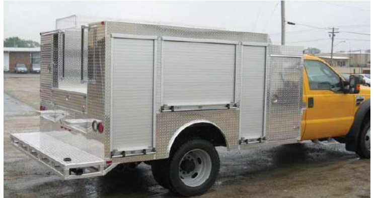
19. One of our most popular set ups. Compartment height at 40" with overhead ladder rack and step bumper. Other popular options include 4" deep flip top compartments on top, adjustable shelving, slide out trays, painted doors and much more. All models available in smooth or treadbrite aluminum construction.
