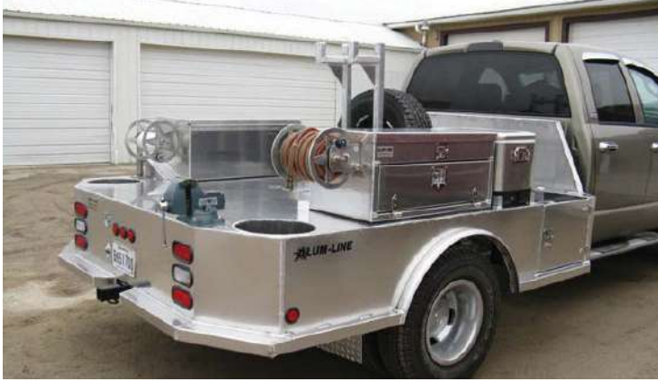
4. Beds can be designed with a frame cut-out to attach special use equipment. Side boxes can be built any height. Beds built tough enough for medium-duty trucks.
