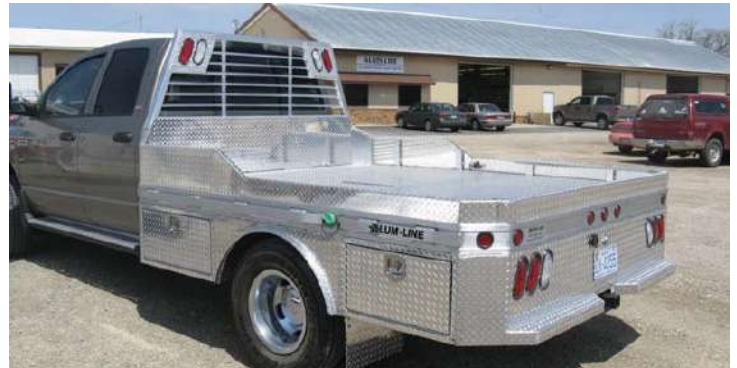
8. Another choice of sides can be matched to almost any inch increment you desire. All hitches used with ALUM-LINE beds are attached to the frame of the truck.
