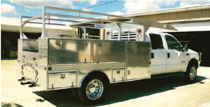
5. Overhead ladder racks can be made permanent or removable. Side boxes are available with double drop-down doors. Large front storage boxes.
