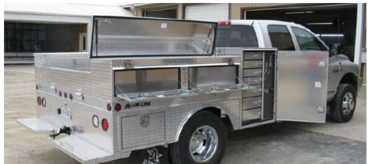
3. Component body. With our special front corner cutouts, you can have tall upright boxes yet the strength of a platform body. Extra storage includes removable top boxes and small boxes behind the wheels. A lower price alternative to a service body.
