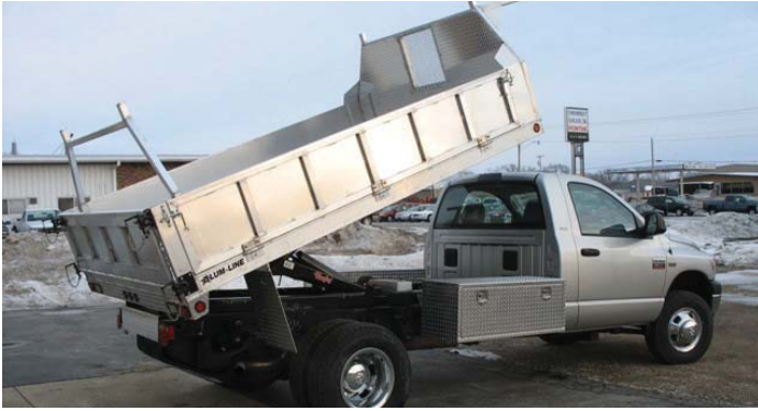
16. ALUM-LINE dump body platforms are heavy duty. Special strength options include; 1/2" thick outside framing with 1 1/4" extruded flooring. Channel long sills and heavy duty bulkheads complete the package.
