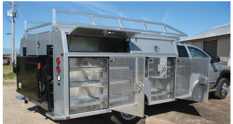
21. All types of customizing available including shelving, transverse compartments, roll out trays, double pan doors, door stops, special latches, hanging hardware, and interior lighting. Our service bodies have been used and approved by the U.S. Army.
