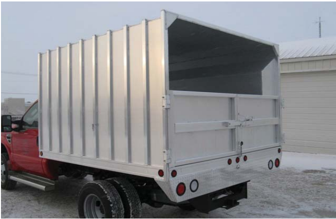
17. Bed capacities up-to 12 ton are available. Our extruded flooring offers easy dumping. Permanent solid sides come in a variety of heights and in either smooth, extruded, or diamond plate material.
