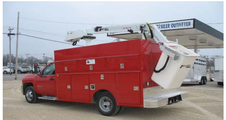
20. Service body with extra height. Multiple compartments per side and finished 1.125 smooth aluminum painted sides. Rear step bumper and rolled fender flares. More information is available on our complete line.
